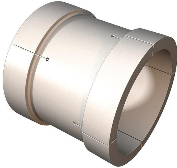
The Castool Clean-out Block has been designed for maximum efficiency in cleaning the liner wall. The block is long enough to sit on the billet loader and travel through the liner smoothly. It is made to be used at room temperature to make handling safer and to achieve better dimensional control. The block is made hollow to reduce weight and wire cut at both ends to allow it to flex slightly and retain contact with the liner wall.
