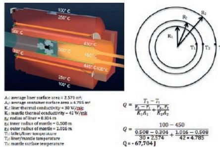
1 Stable thermal gradient of the QR container and its temperatures in different areas.
