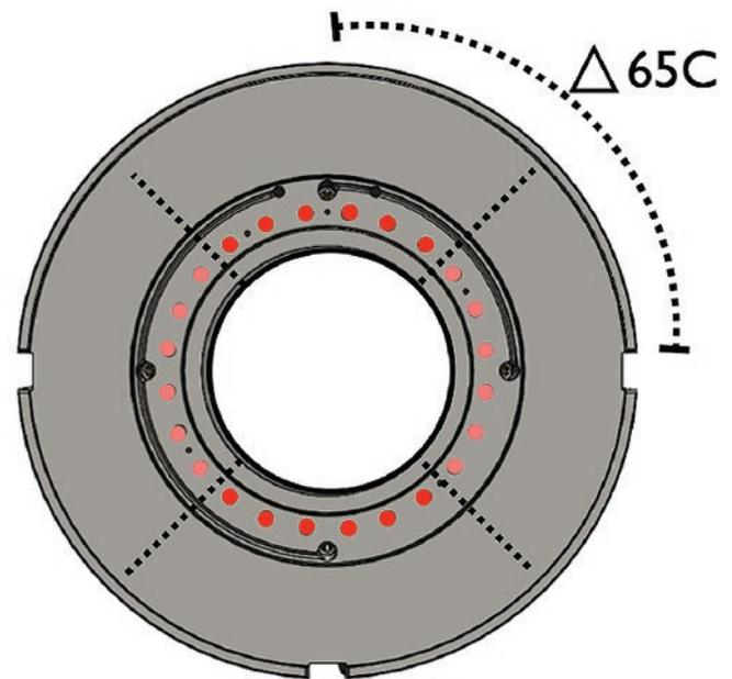
*3 The temperature between adjacent zones could be as high as 65°C on a 12 inch container.*
