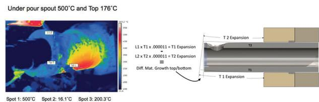
Figure 3 – Shot sleeve distortion due to unequal thermal expansion.
