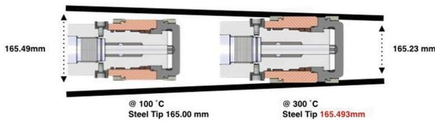
Figure 1 – The plunger tip over expands and sleeve contracts near die end.
