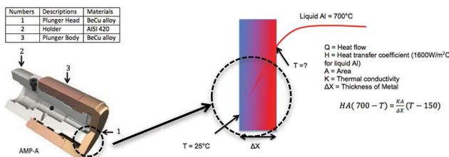
Figure 2 – Heat transfer calculation of a plunger tip.
