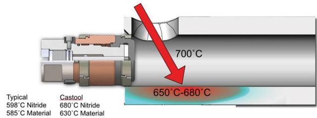
Figure 6 – Thermal stabilities of different shot sleeves and iron nitrides.
