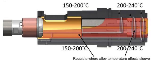
Figure 4 – Thermally regulated shot with optimal sleeve temperature.
