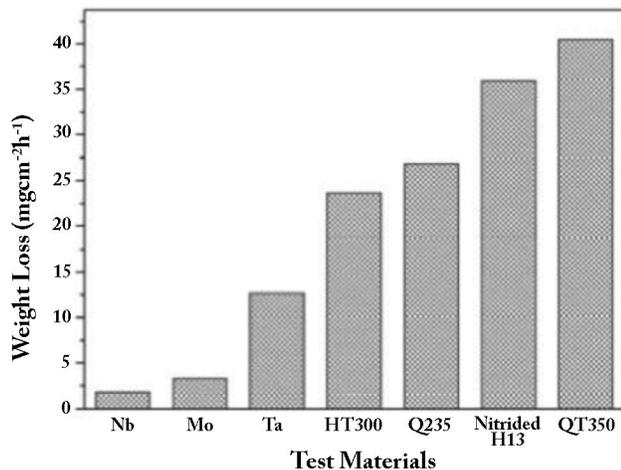
Figure 5 – Corrosion of H13 and molybdenum in liquid aluminum.
