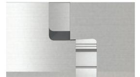
Two pin hoods are now being machined into most rings. The split is kept away from the pour spout and also erosion prone area of the shot sleeve, under the pour spout. The ring complies to the ID of the shot sleeve better than with a single hood opposite the split. It is also easier for the operator to access the split for removing and installing a new ring.
